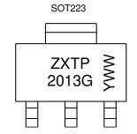
ZXTP 2013G = Product Type Marking Code YWW = Date Code Marking Y or  $\overline{Y}$  = Last Digit of Year (ex: 5= 2015) WW or  $\overline{W}W$  = Week Code (01~53)
